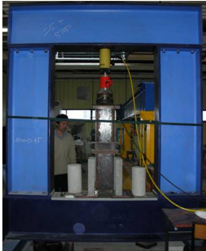
Fig. 2.4 Push-out loading equipment
